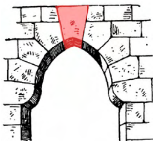
A stone bridge with keystone and voussoir
